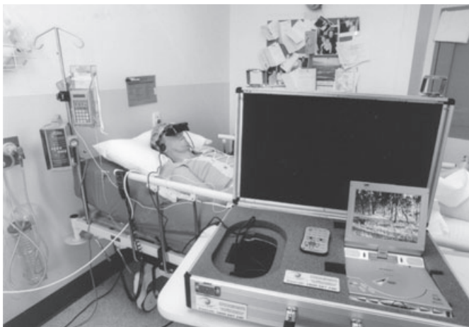
Figure 1. The Virtual Reality Hypnosis System, developed by Virtual Medicine Pty Ltd.
